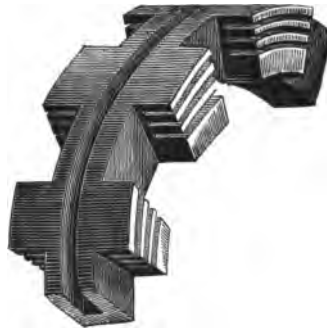
Fig. 81.—Section of Brush's Armature. Earlier (solid) type.
